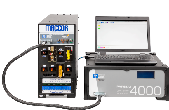
Maccor Model 4300M connected to Princeton Applied Research PARSTAT 4000 Impedance Analyzer
